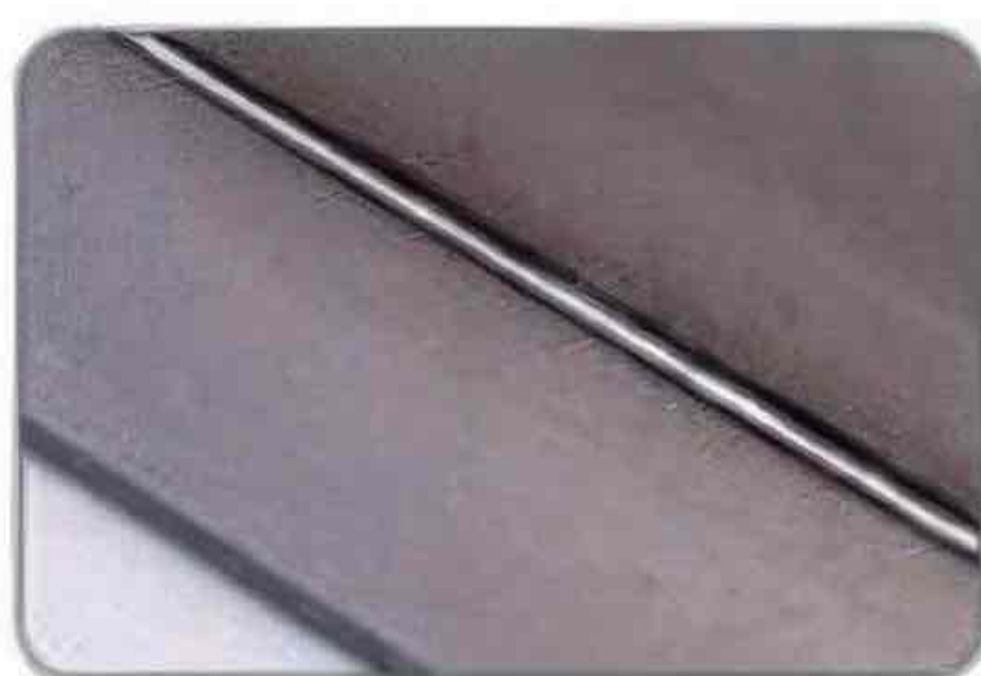
2mm stainless steel fillet welding
