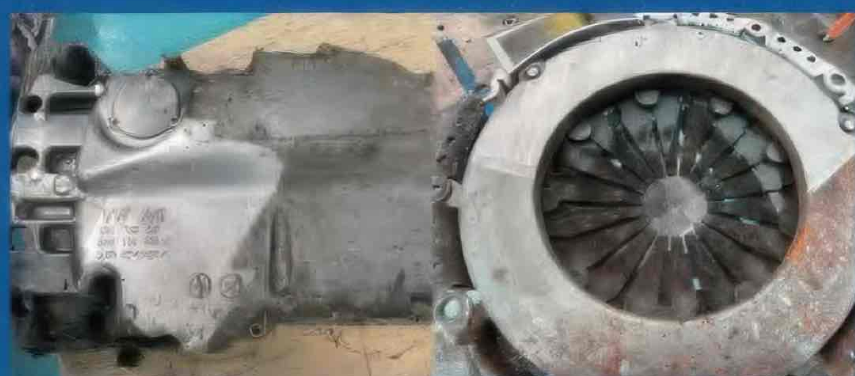
Laser Cleaning Auto Parts
