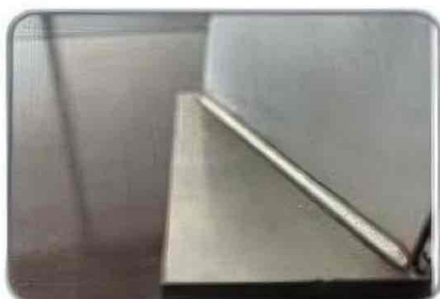
Stainless steel inside fillet welding
